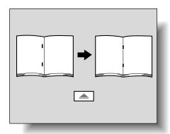
8 If the staple position is too far to the right of the center of the paper, touch to specify the desired negative adjustment (between -1 mm and -7 mm).
